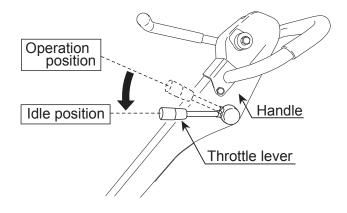
Figure 18. Throttle Lever (Idle)
